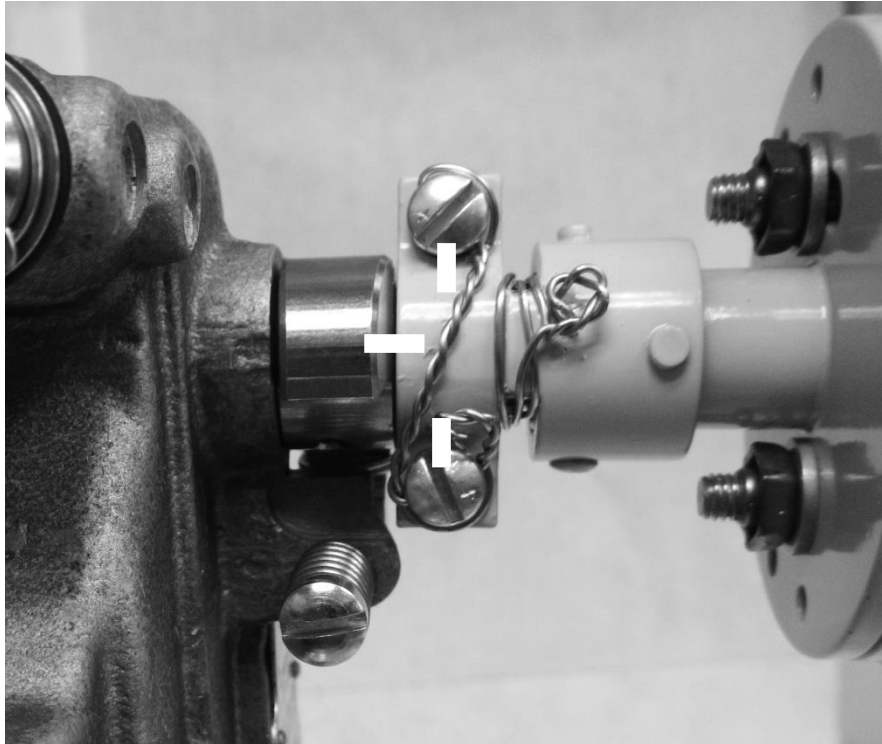
Figure 5-11f: Application of Anti-Sabotage Lacquer
